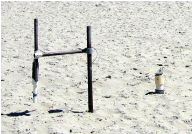
FIGURE 2-7 Photographic image of a Sensit device suspended above the ground (left) and a Cox Sand Catcher (right). NOTE: The Sensit is a battery-powered motion detector used to count sand-sized particles per unit time that saltate (bounce) across the surface. The Cox Sand Catcher is a passive device used to capture samples of wind-blown, sand-sized particles of dust at a specific height above the surface. SOURCE: Richmond, 2019.
