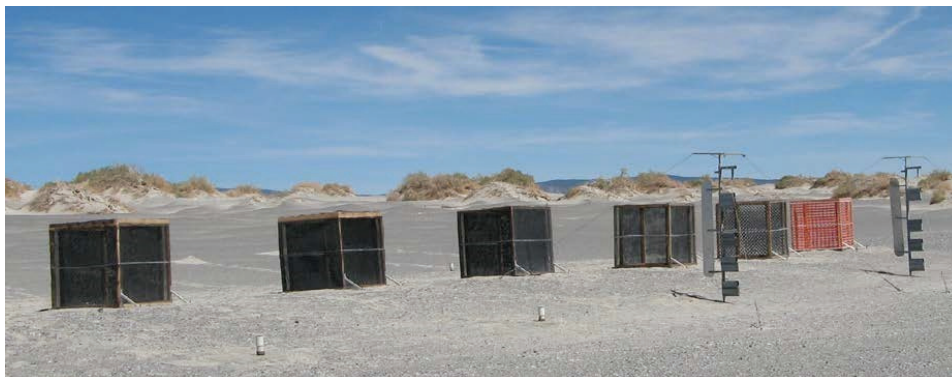
FIGURE 4-11 Testing of engineered porous roughness elements at Mono Lake. SOURCE: Holder, 2019c.
