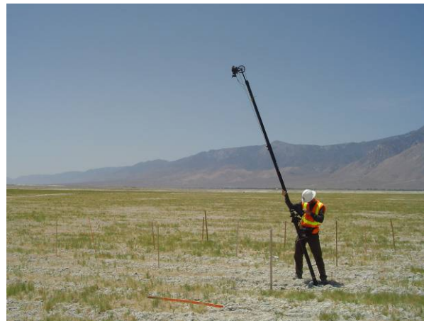
FIGURE A-3 DPF Field Equipment Setup DPF equipment included the use of a high resolution camera mounted on a 15' Hi-Pod monopod.
