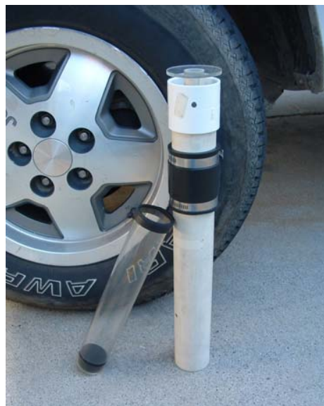
Figure 2.3 - Example of a Cox Sand Catcher (CSC) with the inner sampling collection tube removed.
