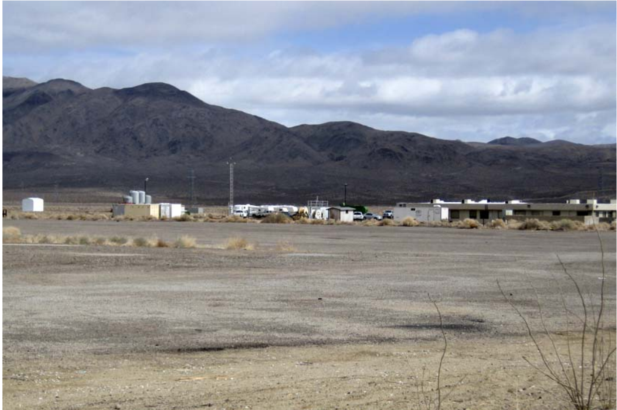
Figure 5. Windblown dust from this truck parking area located west of the PM10 monitor site at the Coso Junction rest area caused two exceedances of the PM10 standard in 2007. The parking area was graveled in 2008 to control dust. In 2009, most of it was paved and used as a staging area for a highway construction project. The PM10 monitor site is the structure with the railing on top in the center of the photo. Coso Junction wind measurements are taken at a 10 m height on the tower to the left (north) of the PM10 monitor. (View looking to the northeast, February 24, 2010)
